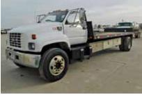
1998 Chevrolet C-7500, 129,013 miles, straight truck, Cat 3116, 215 hp, Dana Spicer fully synchronized 6 speed, 18' bed, 40" frame behind bed, (3) 48"x18"x18" toolbox per side, single 21K rear axle, spring ride, A/C, power steering, air brakes, wet kit, dual 50 gal. fuel tanks, 260" WB, 22.5 LP tires, (4) alum., (2) steel wheels, VIN 1GBM7H1J1WJ101817
