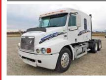
1998 Freightliner CL112, 40" flat top sleeper, Cummins M-11 Eaton Fuller Super "10" Airliner air ride susp., power right hand window, power mirrors, heated mirrors, diff lock, air slide 5th wheel, cruise control, dual air ride seats, dual 100 gal. fuel tanks, Meritor 40K rear ends, 24.5 tires, (10) alum. wheels, VIN 1FUYNMDB1WP715420
