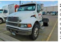
2005 Sterling Acterra, 247,710 miles, day cab tractor, Cat C-7, 250 hp, 7 speed, air ride susp., A/C, dual air ride seats, single 90 gal. fuel tank, single 23K axle, 151" WB, 22.5 tires, (6) alum. wheels, VIN 2FWBCGDC85AV06134
