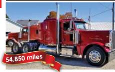
2008 Peterbilt 389, 54,850 miles, 40" unibilt flat top sleeper, Cummins ISX, 550 hp, Performance tuned, Eaton Fuller, 18 speed, flex leaf air ride susp., diff lock, air slide 5th wheel, power windows, power locks, power mirrors, cruise
